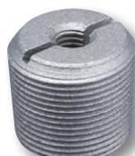
Screws into top of pole with 1-1/4" NPT threading and allows for insertion of ornament with either a 1/2"-13NC or 5/8"-11NC spindle threading.
